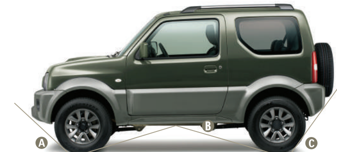
A 34° approach angle (default setting, unloaded Jimny) B 31° ramp breakover angle C 46° departure angle
